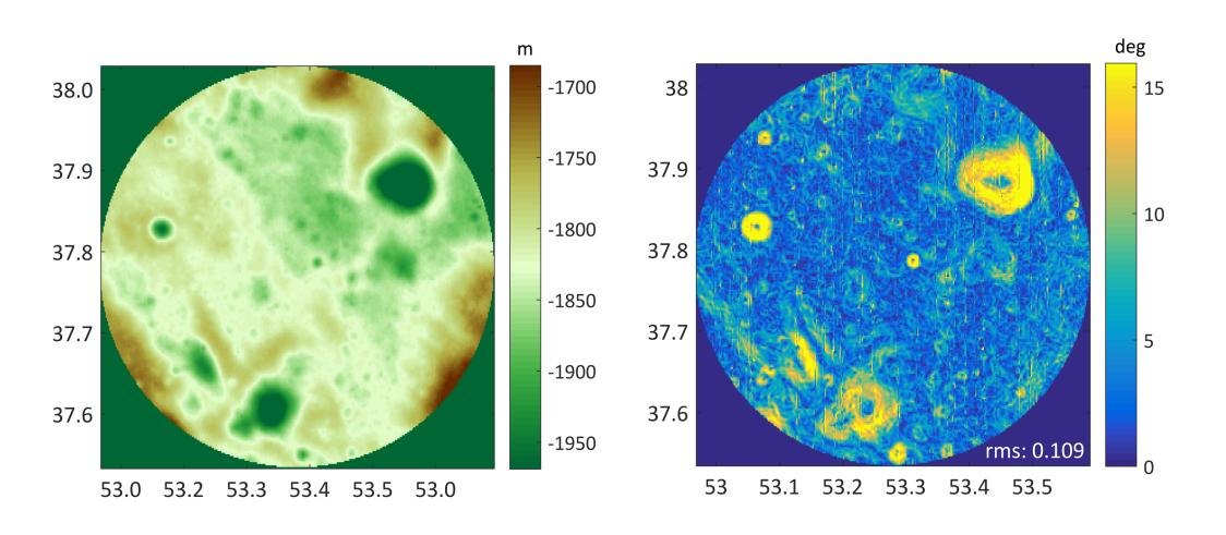
Left - topography from SLDEM in resolution of 512 pix/deg [3]. Right - surface bidirectional slope calculated from the left panel, on scale of ~60 m. Both color bars scaled to 3 sigma range.
