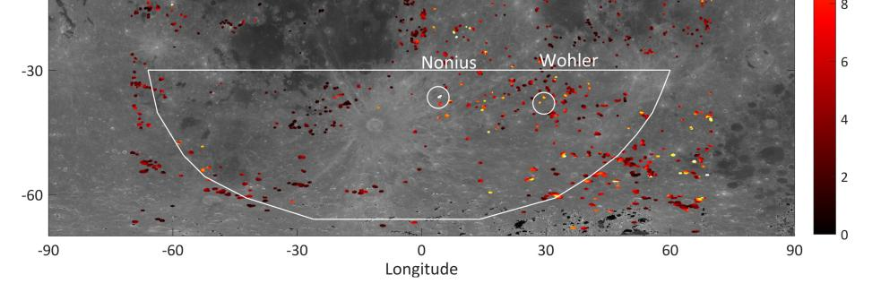
Surface Magnetic Field at Landing Sites: all candidate landing sites on the background of the moon's albedo. Each colored pixel is part of an optional site, while the color represent the magnitude of the magnetic field at the surface. 3 clusters of sites were detailed analysis so far, 2 in the southern hemisphere and 1 in the northern one, as presented below.
